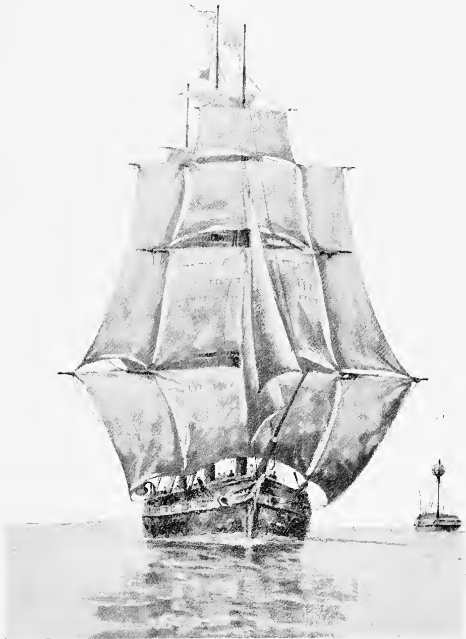
BOW VIEW OF AN OLD BRITISH SHIP, THE CALCUTTA, WITH STUDDING SAILS SET.
